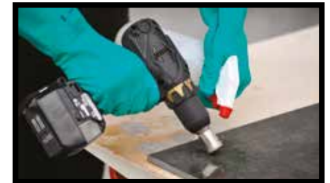
Fig.9/10 - As an alternative, you can use cutting discs fitted to angle grinders, electrical drills or battery-operated screwdrivers.
