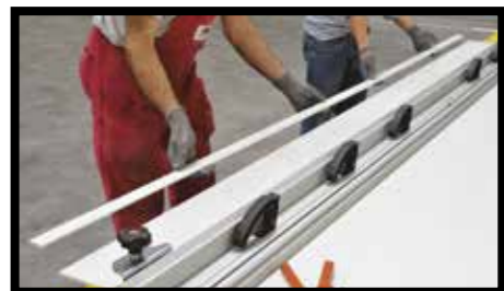
Fig.5 - A practical tool for cutting is the tile cutter ruler (for instance Keracut from Sigma or Free-cut from Raimondi ). As far as ZERO.3 3PLUS and ZERO.3 5PLUS are concerned, after scoring the ceramic part and splitting the slab, complete the operation by cutting the fibreglass mesh with a standard cutter (Fig.4).
