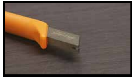
Fig. 1 - You can obtain excellent results in terms of shaping and clear cuts by scoring all versions of ZERO.3 with Silberschnitt 2000 special glass cutters produced by Bohle Italia or with the manual tile cutter produced by Würth . To achieve good cuts, throughout the entire cutting operation never detach the glass cutter from the tile.
