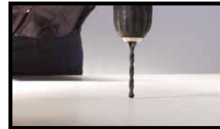
Fig.8 - As far as manual drilling is concerned, use tungsten bits with a diameter up to 10 mm, fitted to electric drills or battery-operated screwdrivers.
