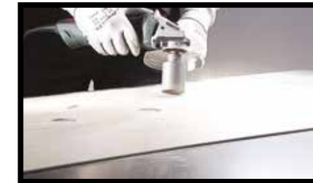
Fig.9/10 - As an alternative, you can use cutting discs fitted to angle grinders, electrical drills or battery-operated screwdrivers.
