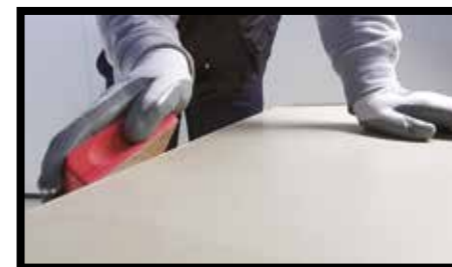
Fig.12 - Edges can be finished by hand using abrasive diamond sponges or emery paper. With a light passage on the side of the slab, you can obtain a slightly rounded-off edge or with repeated passages a bevelled effect.
