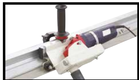
Fig.6 - With tile cutter rulers, you can use hand-held angle grinders, fitted into special frames that can be "fit onto" the cutting guide. In this manner, you can provide both 90° and 45° cuts to obtain bevels and jolly pieces.
