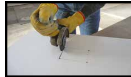
Fig.11 - To obtain internal and L-shaped corners, round off the vertex of the internal corner using bits with a radius of at least 5 mm that reduce the risk of breakage. Then cut with diamond discs, taking care to stop moving the cutting tool forward when you reach the hole previously drilled. To drill and cut using diamond discs, follow the instructions provided above.
